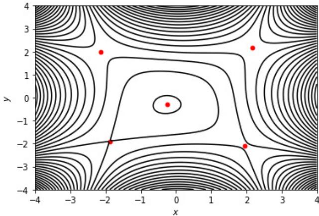
Fig. 1. The contours of the asymmetric Caldera potential (2) with parameters  $c_1 = 5, c_2 = 3, c_3 = -0.3, c_4 = 2.5$ . We depict the positions of the five equilibrium points (one central minimum and four index-1 saddles around it) using red points.
