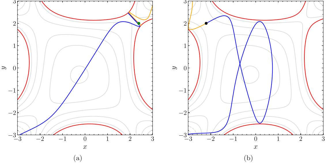
Fig. 10. (a) The forward (blue color) and backward in time (yellow color) evolution in the configuration space ( $x, y$ ) of the trajectory denoted by a green point in Fig. 9. (b) Similar to (a) but for the trajectory denoted by a black point in Fig. 9. In both panels, red curves depict the boundary of the energetically forbidden region.
